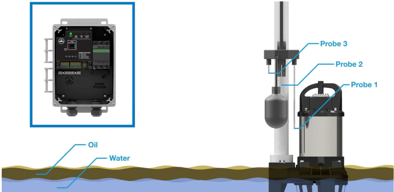
Conductive probes monitor oil and water levels, allowing the Oil Watch™ system to pump out water while keeping oil contained in the sump pit.
